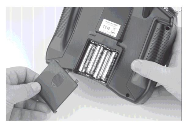
This view of Spectrums' new 5 channel transmitter shows it's made for economy. The four cells probably work OK, but I hope those battery clips are sturdy or you've got problems.
